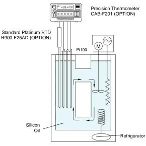
When comparison calibration of glass thermometer, then Pt 100 in above is changed to glass thermometer. Also wire connection from glass thermometer to CAB-F201 is removed.
