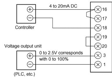
\* Output of voltage output unit needs to be insulated to connect multiple units (JW). A voltage output unit can not be connected in parallel to multiple units.
