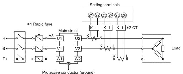
\*1 For models without the rapid-break fuse, make sure to connect a rapid fuse externally to protect a system.
