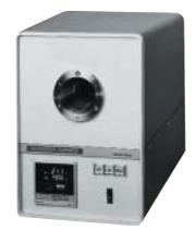
The black body furnace for medium temperature range is used for comparison calibration by utilizing a fixed-point calibrated  $0.90\,\mu\mathrm{m}$  silicon monochromatic radiation thermometer as the standard thermometer, and the black body furnace for low temperature is used for calibration by utilizing a optional built-in platinum resistance thermometer as the standard thermometer.
